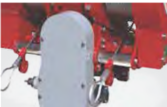
Robust Rollers for directing of wire rope
