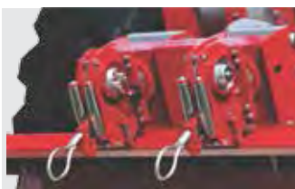
Compact Driven Pulleys allow free rotation and help when extracting the rope from the drum and ensure solid and even rope coiling.
